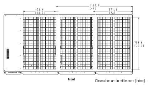
Figure 3-7. UPM Section Dimensions (Top View)
